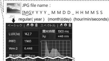
▲ You may save measurement screen in "BASIC mode", "SPECTRUM mode", "PPFD mode", "PFD mode" and "CIE 1931.1976 mode".
