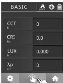
Press the measurement button at bottom center of screen or the measurement key at left hand side to measure. (You can press measurement key at both sides.)
